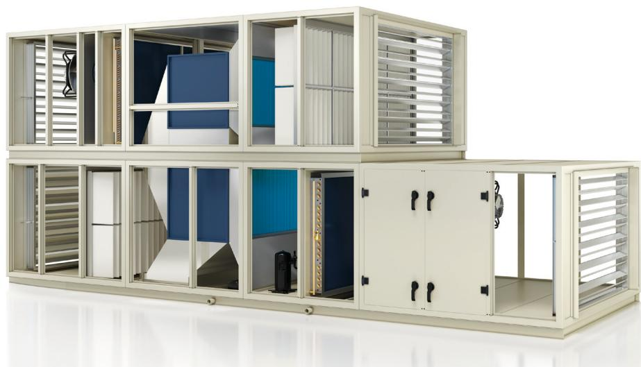
In very hot climates, DX cooling is added to the existing system. The complete DX system with compressor, evaporator and condenser is also housed inside the unit. With this enhancement, 30 % of the required cooling can be generated mechanically. In this way, the system can be used in practically any climate zone.
